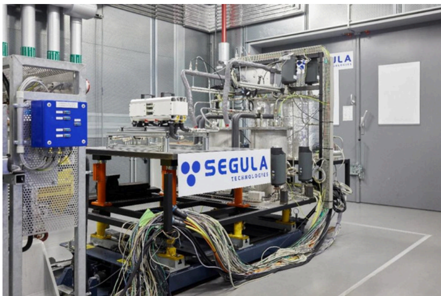
Figure 3: A fuel cell stack on the test bench. © Segula Technologies
